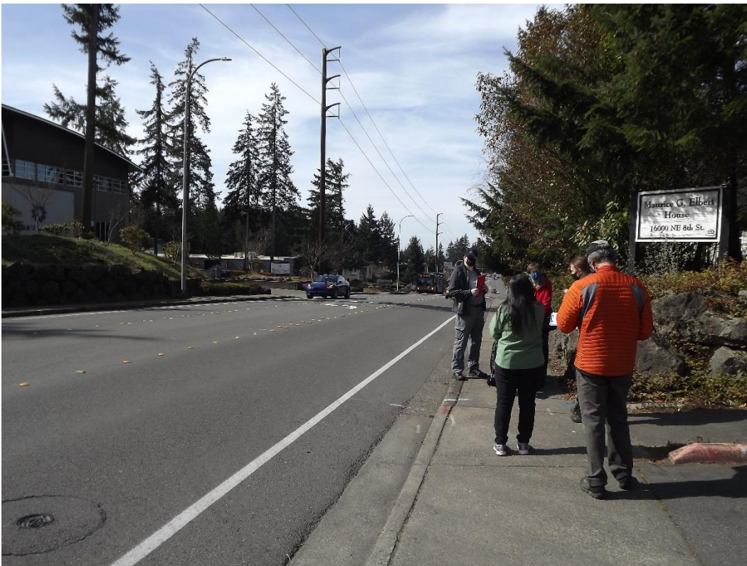
Left: Our group stops at the site of a pedestrian fatality in November 2020 and reflects on the road design elements that contributed to this collision. The nearest marked & signalized crosswalks were several hundred feet away – an added distance that can be inaccessible for mobility-challenged residents.
